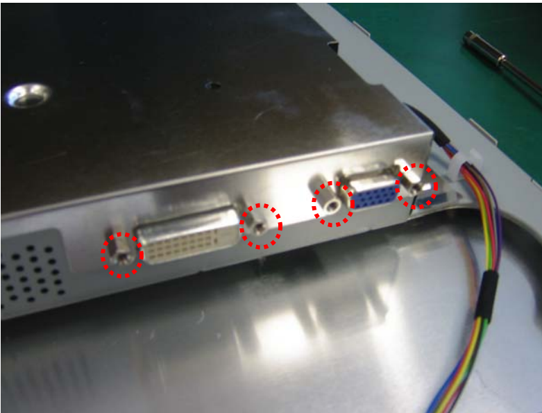
F. Fix the main shielding by connector screws.
